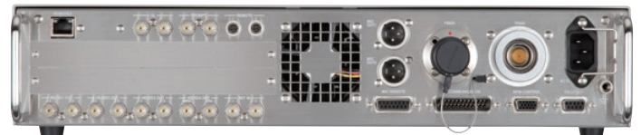
CU-HD1300FT Rear Panel (Fiber/Triax)
